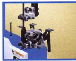
Upper and lower ball bearing blade guide system
